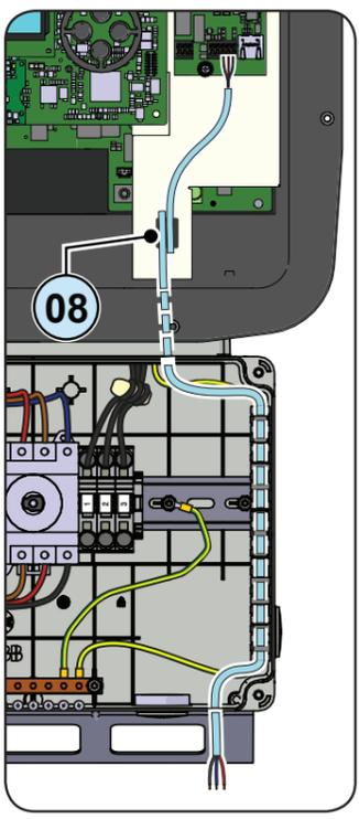
To connect the wires to the Alarm 04, RS485 and REM 06 connector terminals:
