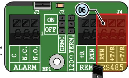
The last inverter of the daisy chain must be "terminated". Apply the 120 Ohm termination resistance by configuring the RS485 Line Termination Jumper 02 to the "ON" position.
