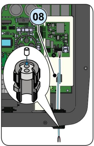
**CABLE CONNECTION IN INVERTER VERSIONS WITH WIRING BOX**
