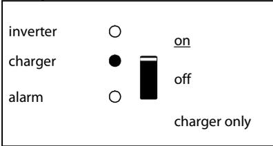
The AC input voltage is switched through and the charger operates in bulk or absorption mode.
