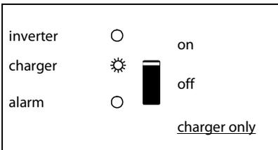
The AC input voltage is switched through and the charger operates in float mode.
