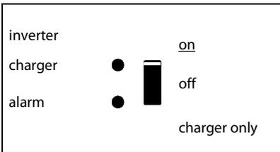
The AC input voltage is switched through and the charger is switched off.
