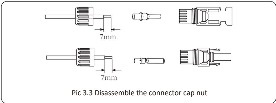
Pic 3.3 Disassemble the connector cap nut
