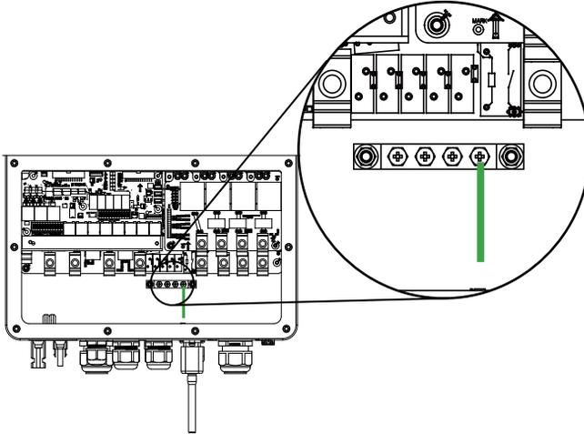
Earth connection(Copper wires)
