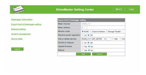
(3) In the third drop-down list, fill in the communication address of monitored device
