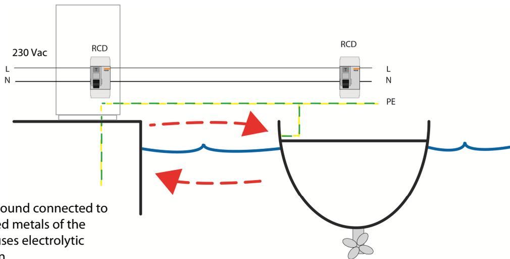
Shore ground connected to immersed metals of the boat causes electrolytic corrosion
